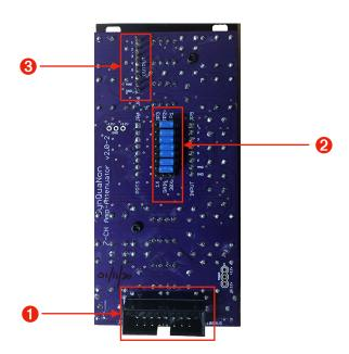
1 A100 Bus Keyed power connection with reverse polarity protection.
